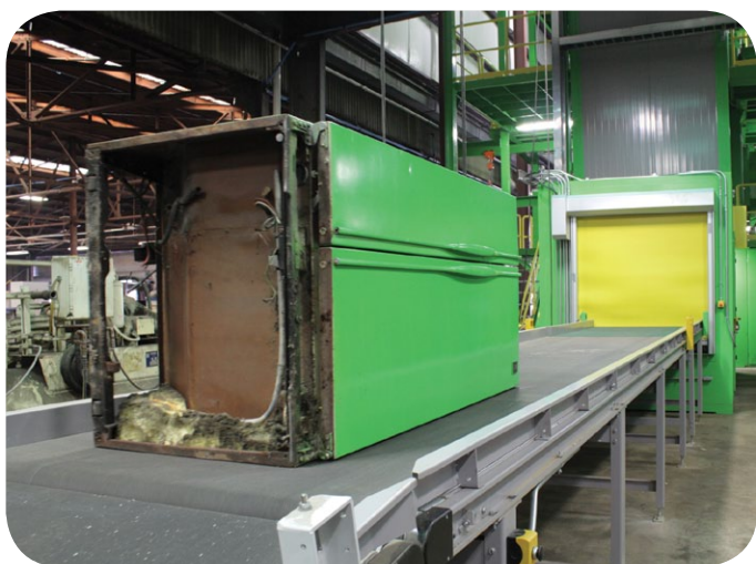
The URT system can process approximately one refrigerator per minute. GE, in collaboration with ARCA, reached a milestone of 100,000 refrigerators and freezers recycled. Photo: GE Video: www.youtube.com/watch?v=ugjRbw1-iU8
